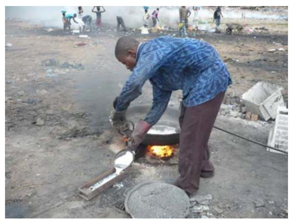
Figure 3 Lead refining from battery scrap with open fire in Ghana (photo Öko-Institut e.V.)
