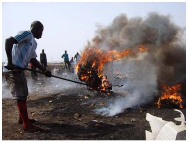
Figure 2 Cable burning with open fire in Ghana (photo Öko-Institut e.V.)
