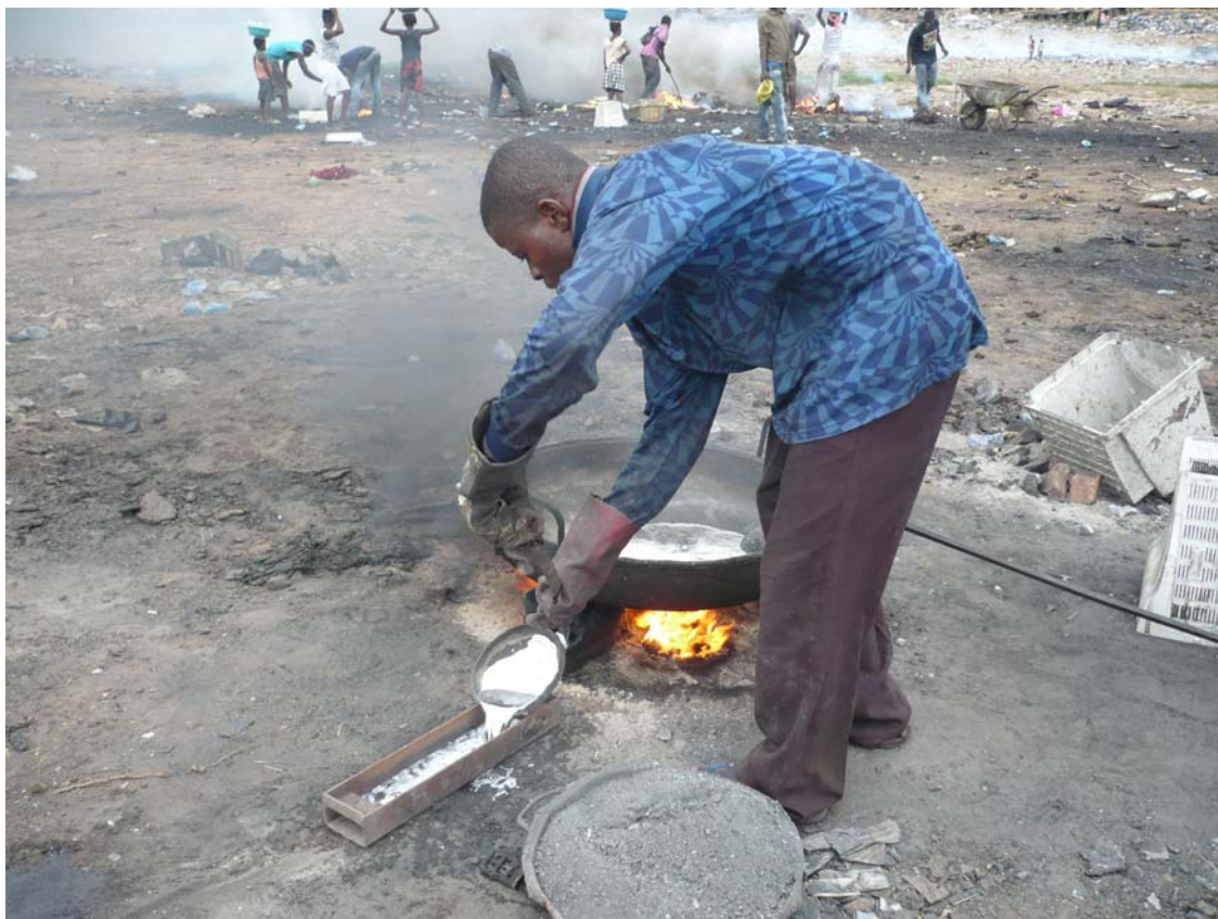
Figure 3 Lead refining from battery scrap with open fire in Ghana (photo Öko-Institut e.V.)
