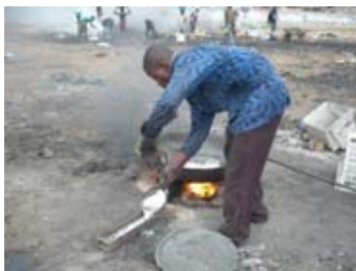
Figure 3 Lead refining from battery scrap with open fire in Ghana (Öko-Institute e.V.)
