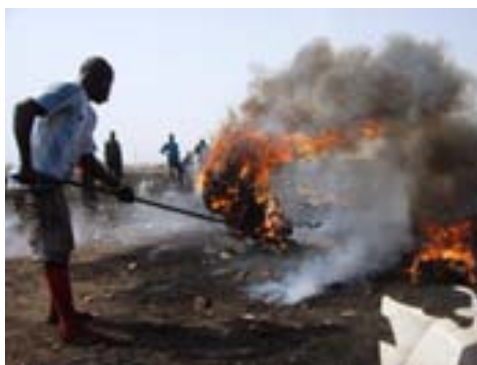
Figure 2 Cable burning with open fire in Ghana (Öko-Institute e.V.)
