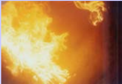
INSIDE VIEW OF INCINERATOR BED AT WORK TEMPERATURES IN THIS REGION ARE IN EXCESS OF 1000°C
