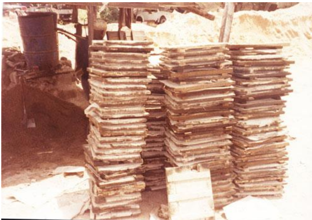
Fig. 4.3b: Pallets treated with used oil in block making
