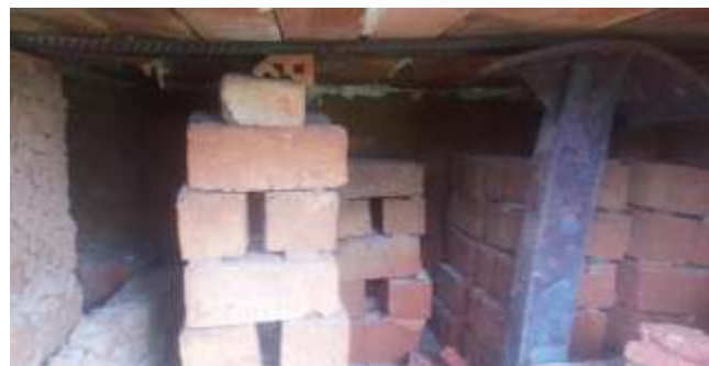
Plate 4: Firing of commercial size bricks in a local ceramics/brick making outfit
