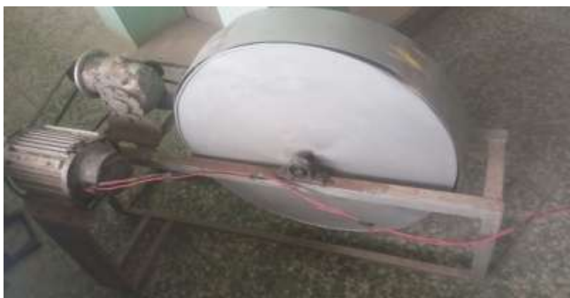
Plate 2: Locally Fabricated Rotary Shaker (28 rpm)
