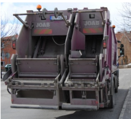
Figure 14. Waste truck with two compartments. Source: private.
