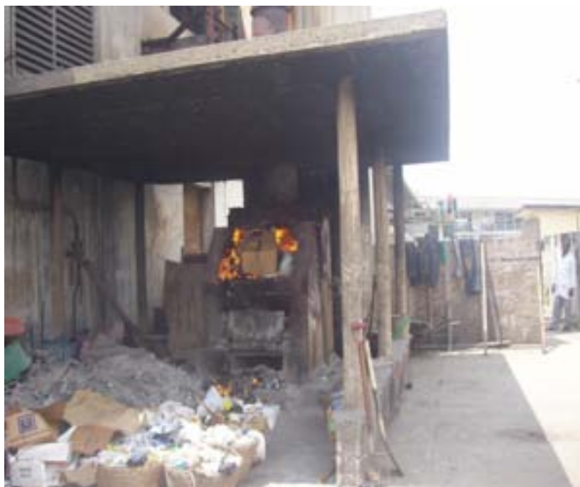
Figure 19 A locally built incinerator at one of the healthcare facilities in Ibadan (Source: Oketola et al., 2011).
