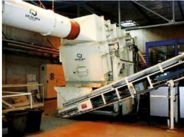
Fig. 21: Waste sorting machine designed by TRISELEC.
