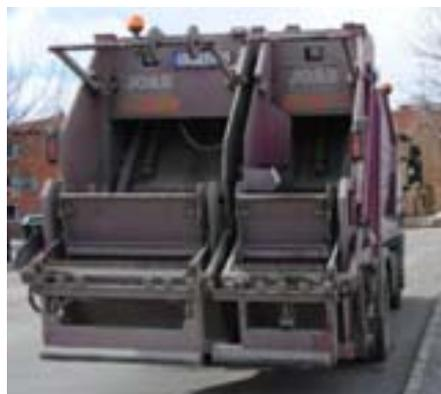
Fig. 16: Waste truck with two compartments. (Private)
