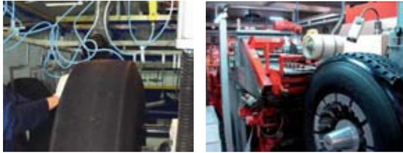
Fig. 11: Re-grooving process
