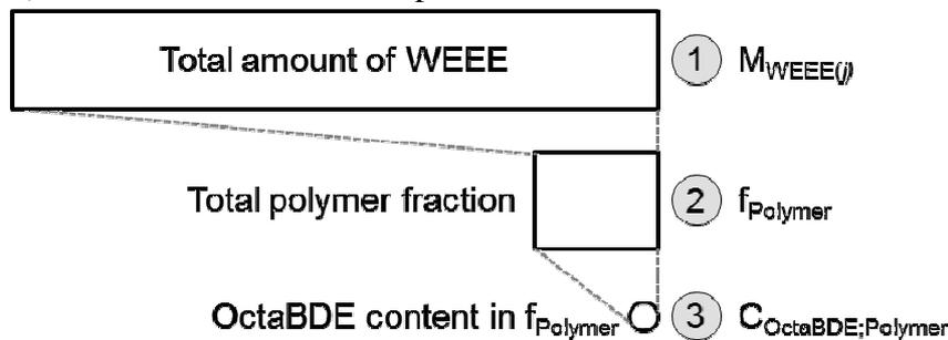
**Figure A-:** Scheme to estimate the amount of c-OctaBDE in EEE entering the waste stream (WEEE)
