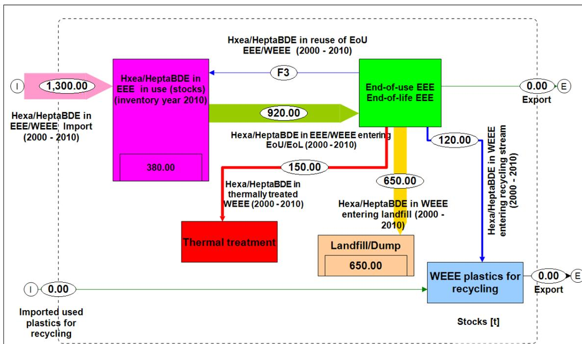
**Figure A-7:** Substance flow of POP-PBDE (tonnes) in WEEE/EEE polymers in Nigeria in polymers of EEE categories 3 and 4 including CRTs and non-CRT equipment (Tier 3 with factor from Nigerian measured data) (Sindiku et al. 2011, 2012)<sup>18,19</sup> (considering the years 2000-2010 in flows<sup>25</sup>; stocks of inventory year 2010).
