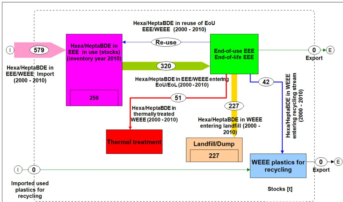
**Figure A-4:** Substance flow of POP-PBDE (tonnes) in WEEE/EEE polymers in Nigeria in polymers of EEE categories 3 and 4 including CRTs and non-CRT equipment (Tier 2 with factor from *POP-PBDE Inventory Guidance*<sup>8</sup>; considering the years 2000-2010 for flows<sup>25</sup>; stocks for the inventory year 2010)
