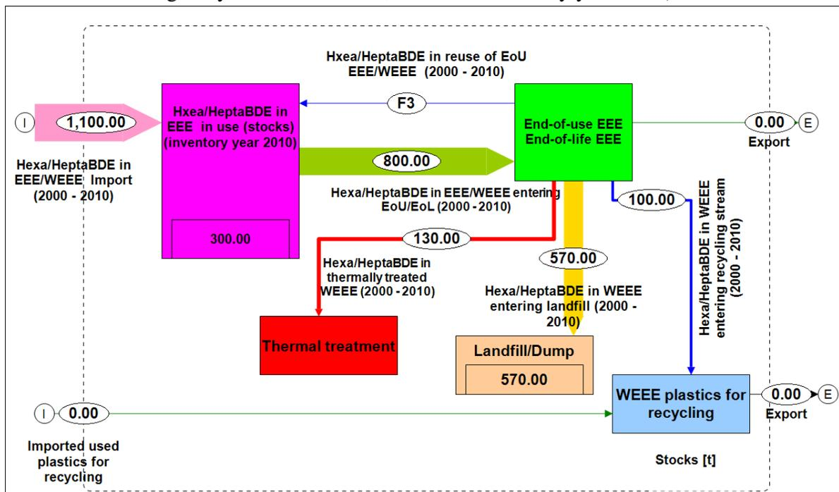
**Figure A-6:** Substance Flow of POP-PBDEs (tonnes) in CRT polymers in Nigeria (with factor from Nigerian measured data; Tier 3) (Sindik et al. 2011, 2012)<sup>18,19</sup> (considering the years 2000-2010 in flows<sup>25</sup>; stocks of inventory year 2010).
