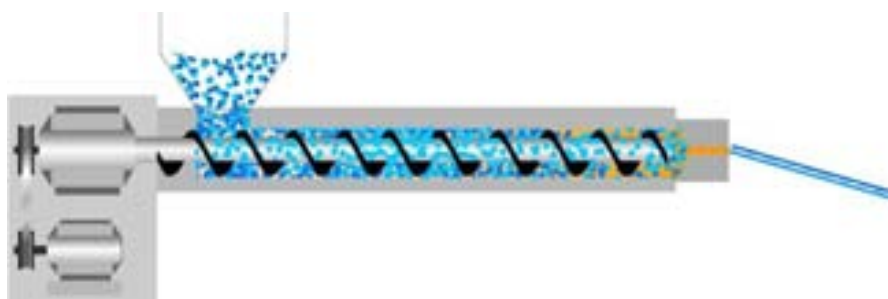
Fig. 11: Plastic profile manufacture by extrusion (source: www.anaip.es )
